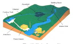
Fig. 10. Hydro Power Plant.
